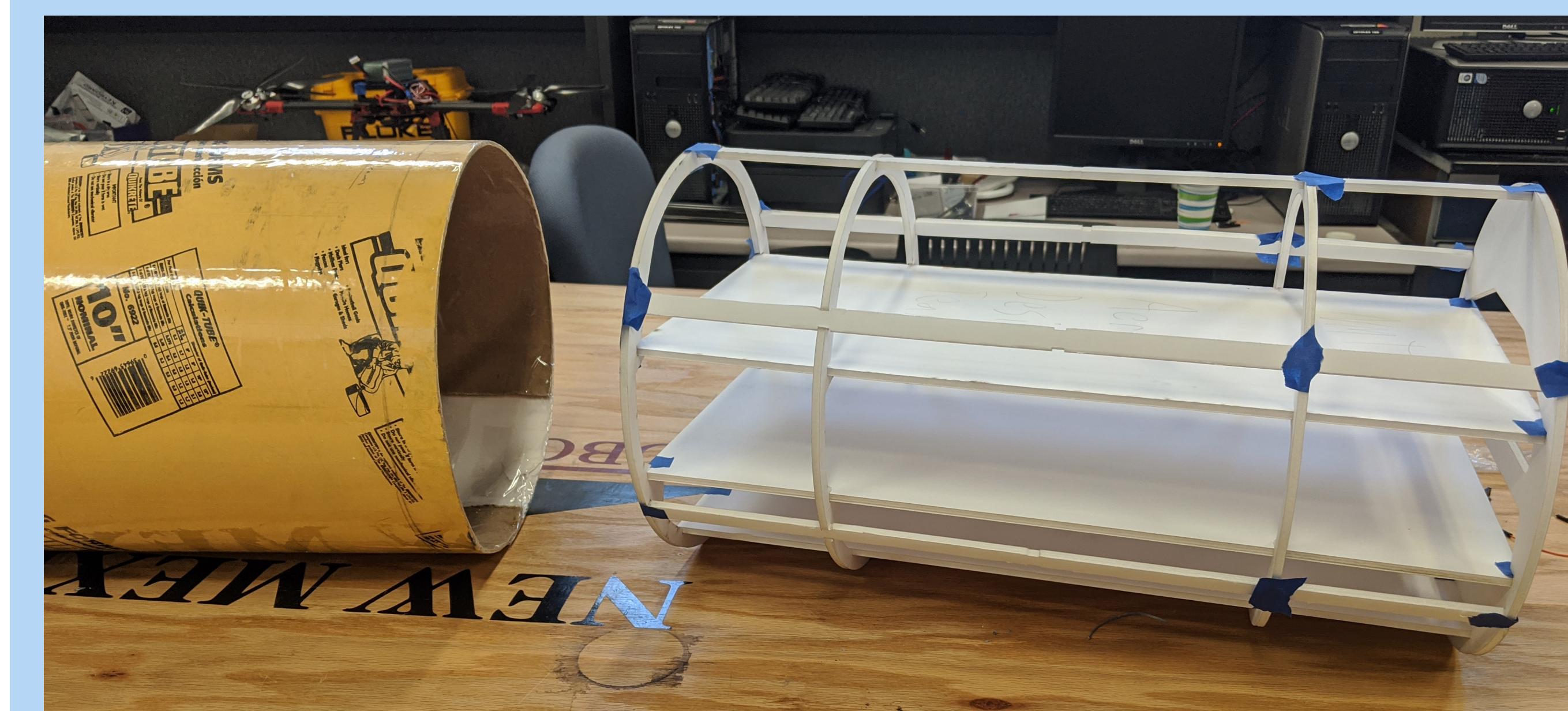
The mold in which fiberglass will be applied too and the interior cargo structure cut from foamboard
