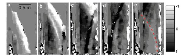
Fig. 9 Contour images from the image correlation processing of test 1. The image region is the same as shown in Fig. 3b. **a** The primary shock wave propagating from *left* to *right*, approaching then  $(\mathbf{b}, \mathbf{c})$  reflecting from the wall with the pressure gages. The primary shock then  $(\mathbf{d})$
