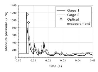
Fig. 7 Measured pressure as a function of time for test 2 at pressure gage locations 1 and 2. The optical measurements are shown as the data symbols and are positioned at the time recorded, measured by the camera frame rate. The optical measurements have an error of approximately  $\pm 50$  kPa
