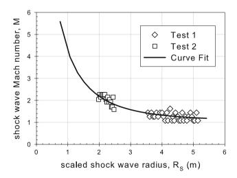
**Fig. 5** Mach number versus scaled radius for C4 showing both experimental data and the curve fit representation of the data. The error in measured radius is less than the symbol size. The error in measured Mach number is approximately two times the symbol size
